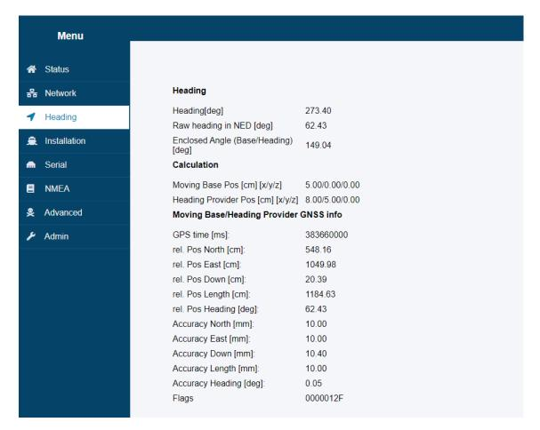
Figure 13: GNSS receiver - Heading page
