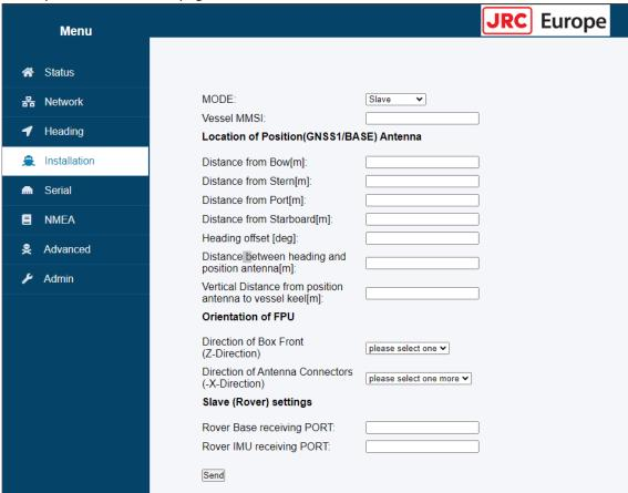
Figure 11: GNSS receiver - Installation page - Slave (Rover) settings
