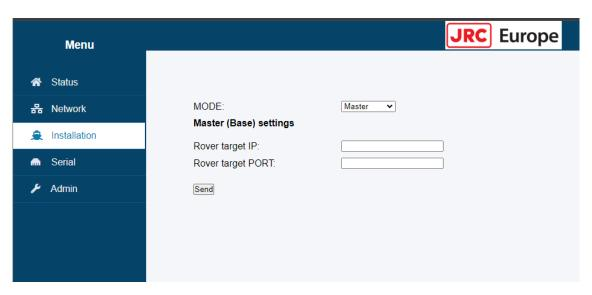
Figure 12: GNSS receiver – Installation page – Master (Base) settings
