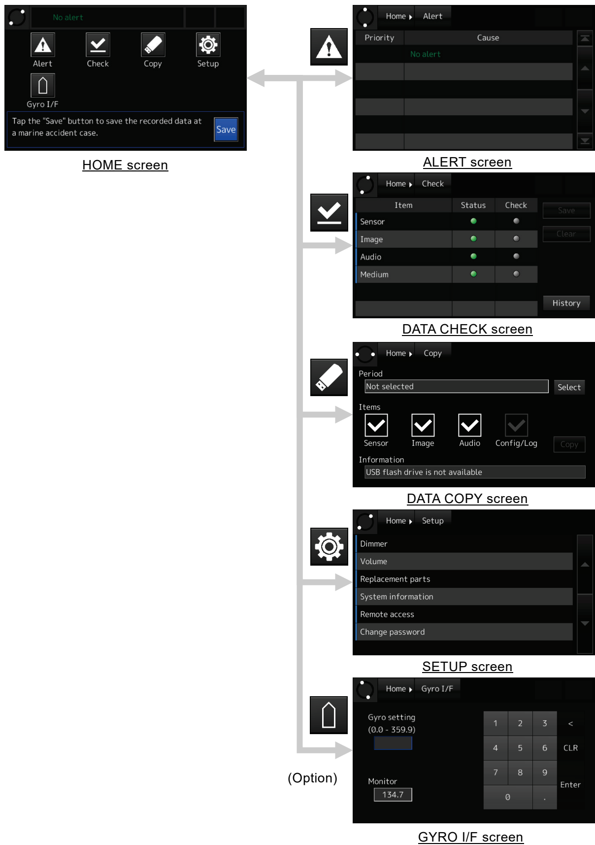
Figure 4-9 Screen transition from the HOME screen
