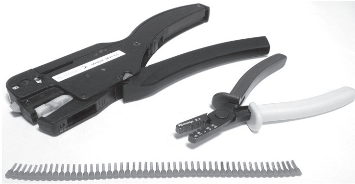
Examples of proper tools for crimping end caps, and a strip of end caps
