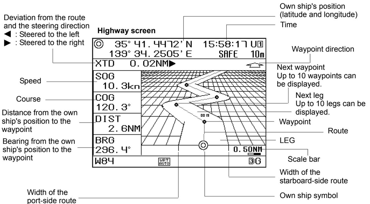
The highway screen's scale can be changed by pressing or . The scale width is the same as the plot screen's. Please refer to "4.3.3 Zooming the Screen In and Out". When GC is selected as the distance calculation method, only one waypoint can be displayed.
