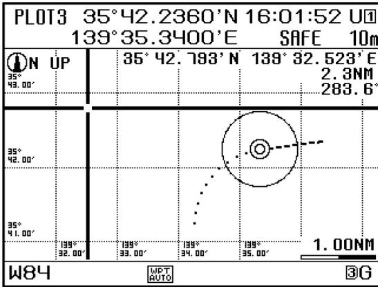
This screen graphically displays the own ship's position in full-screen mode.
