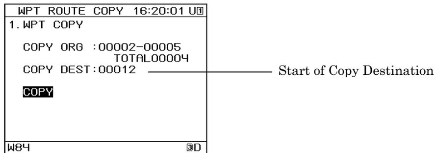
If there is insufficient continuous free space at the copy destination, the following will be displayed. Press **▲** **▼** to select the copy method, and press **ENT**.
