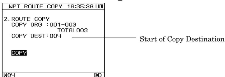
If there is insufficient continuous free space at the copy destination location, the following will be displayed. Press **▲ ▼** to select the copy method, and press **ENT**.
