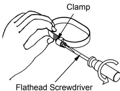
2. Coil the fitting belt around the mast as shown below.
