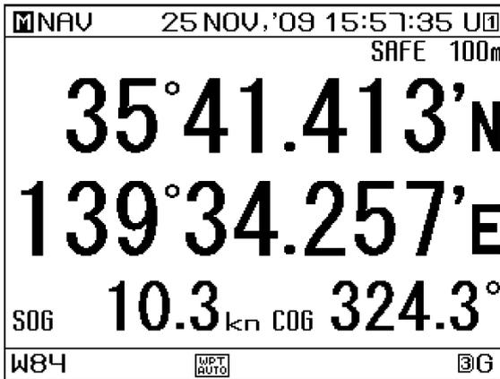
This screen displays information such as the own ship's position. The sub-screens can be displayed by pressing **◀** and/or **▶**.
