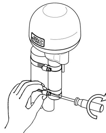
How to Install the Sensor on the Mast
