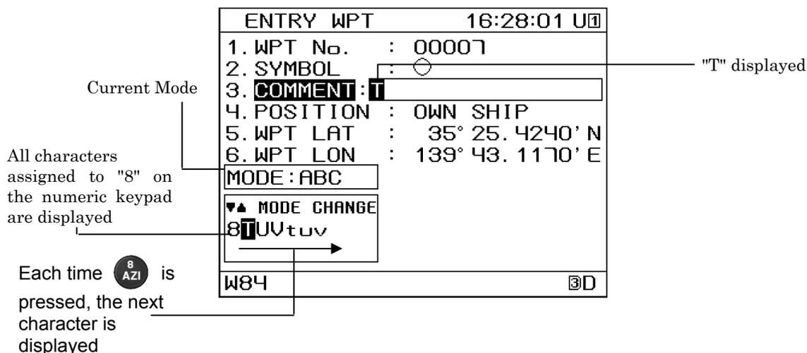
6. The "o" in "Tokyo" is assigned to numeric keypad number 6, so press
