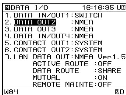
If "SWITCH" is selected when the LAN mutual monitoring mode is set to "OFF", the screen at right will be displayed and the mutual monitoring mode will be set to "ON".
