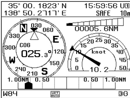
This screen graphically displays the CDI, course, speed, and leg. The highway screen can be displayed by pressing ◀ and/or ▶.
