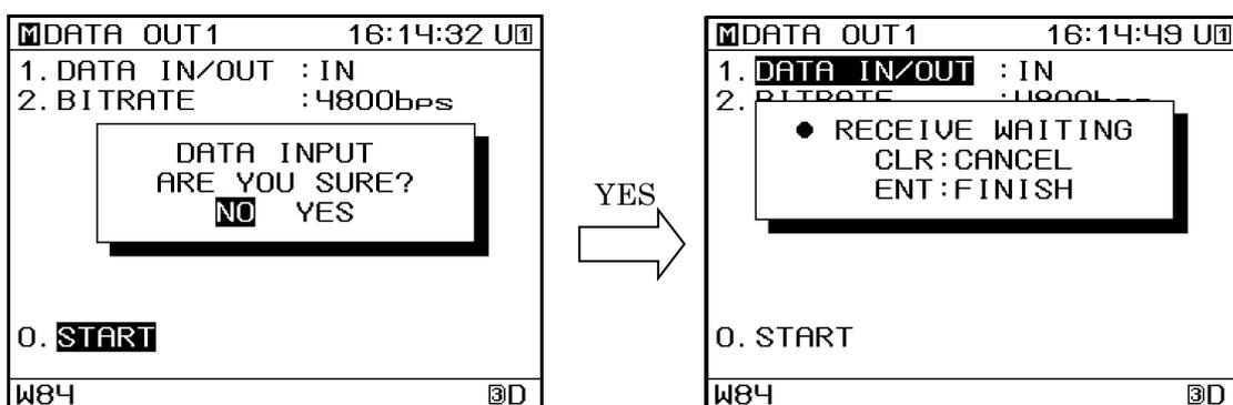
7. Once the unit is awaiting data reception, send RTE or WPL sentences from externally connected equipment. Received data is stored in the internal memory.
