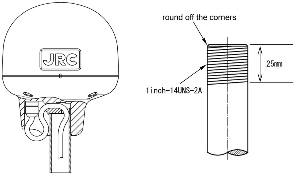
(4) When performing attachment, always hold and turn the sensor base. Holding and turning the radome may result in a large amount of force applied at the junction of the base and the radome, resulting in damage to the sensor. When performing attachment, do not use adhesive for screw or other adhesive for screw part. Adhesive component may attack to the radome, resulting in cracks.
