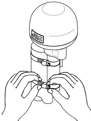
3. Tighten the clamp screw with the screwdriver.
